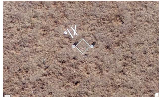
Fig. 2. Visible light image captured during UA flight. White circles are upturned buckets of identical height with rims touching the soil surface. A PVC metre square frame outlines the vegetation sample. Vinyl panels are arranged to identify the sample location. A virtual transect crossing the frame between buckets is used to determine average vegetation height of the sample during analysis.
