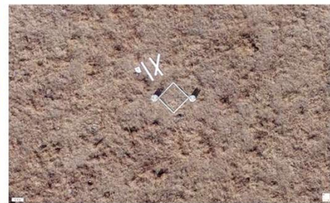
Fig. 2. Visible light image captured during UA flight. White circles are upturned buckets of identical height with rims touching the soil surface. A PVC metre square frame outlines the vegetation sample. Vinyl panels are arranged to identify the sample location. A virtual transect crossing the frame between buckets is used to determine average vegetation height of the sample during analysis.
